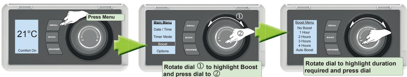
Auto Boost will automatically use the boost element to maintain the set temperature during 'Comfort On' periods.
